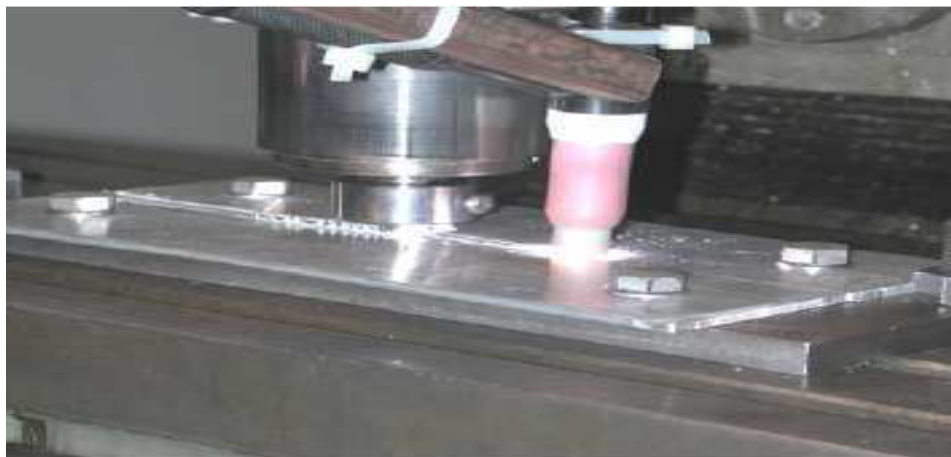
Obr. 4 HFSW zariadenie s participáciou GTAW zdroja ohrevu [14]
